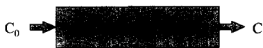
Fig. 2. A schematic diagram of the dispersion flow model with constant velocity, constant dispersion behavior, and constant concentration profile across the tube diameter.
